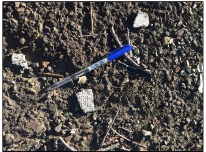
Plate 16 – ACM fragments on asphalt north of the shed.
